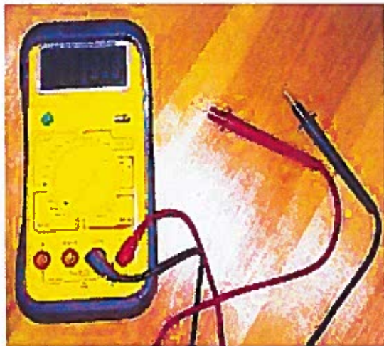
Multimeter set to measure resistance (ohmmeter)
